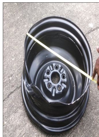
Figure 2: Partly deformed wheel that caused the injuries
